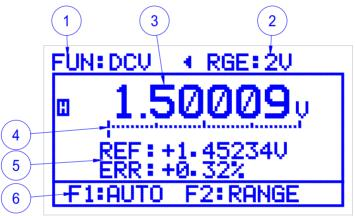
[Figure 10] LCD Display Screen
