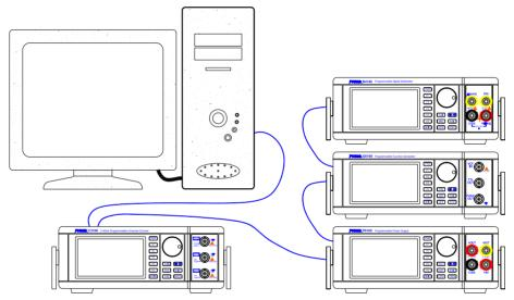
[Figure 4] GP-IB (Example of connecting the connector)
